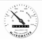
The McCrometer Propeller flowmeter comes with a standard instantaneous flowrate indicator and straight-reading totaliser.
